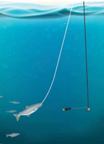
Clip your fishing line to the Downrigger line using a Scotty Power Grip line release.
